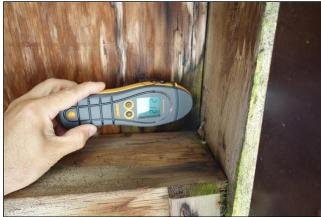
E. (1) High relative moisture reading on front deck.
